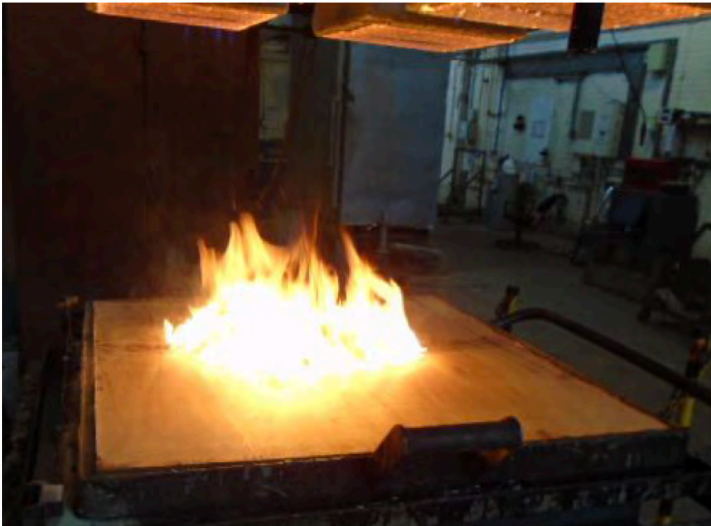
Figure 5- flaming shortly after ignition with pilot flame at 5-6 minutes.
