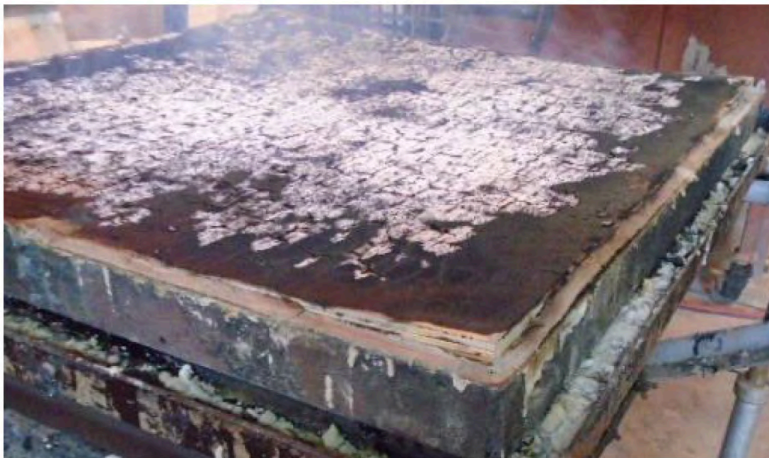
Figure 7- showing edge seal failure.
