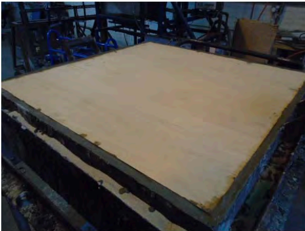
Figure 3- plywood specimen as installed prior to testing.
