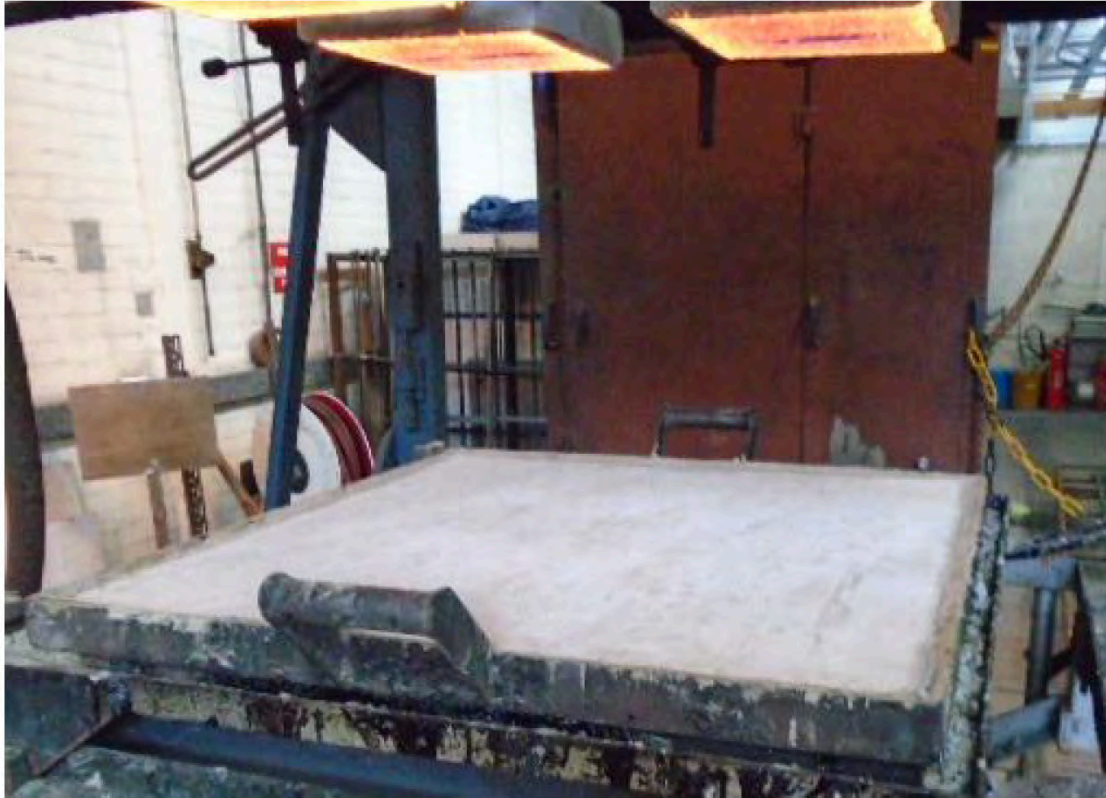
Figure 19- Test specimen 1 at end of 60 minute test.
