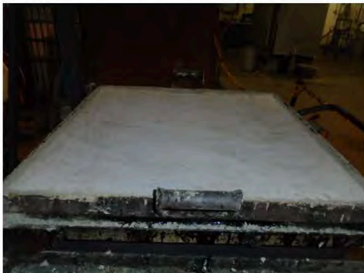
Figure 21- Test specimen 2 at end of 60 minute test.
