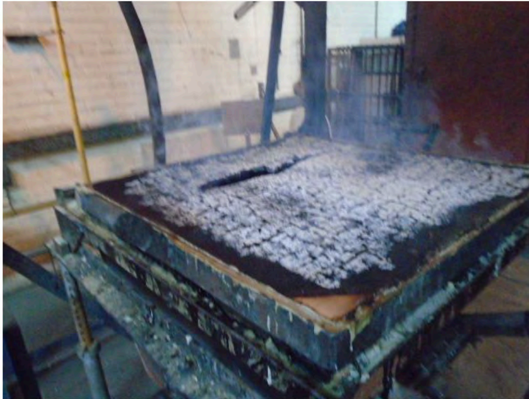
Figure 9- showing the failure at 40 minutes.
