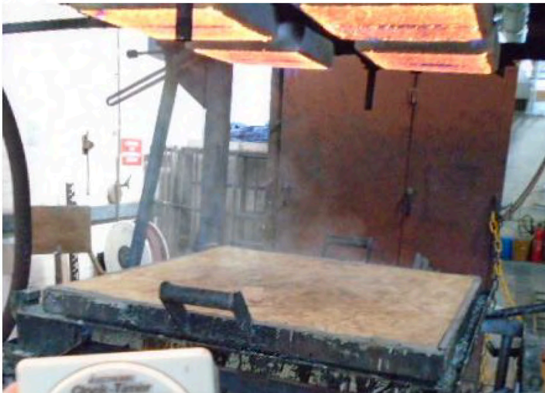
Figure 15- Test specimen at 4:25 minutes, prior to ignition.
