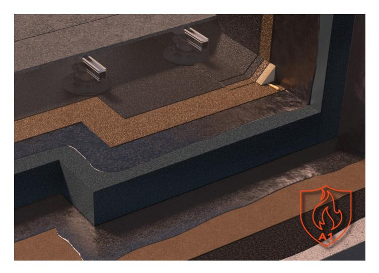
A warm roof insulation board manufactured from specially graded recycled glass ( $\geq$  60%) and natural raw materials.
